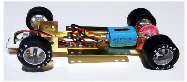
H&R Racing Products Adjustable Wheelbase 1/24 RTR assembled Rolling Chassis -Wheelbase adjustable from 3 5/8" to 4 7/8" (92mm to 123mm) - Includes new 40,000 RPM Motor with larger cooling holes, Rubber rear tires on setscrew aluminum hubs, rubber front tires on setscrew aluminum hubs, Oilite bushings, body mounting kit - Comes with inline motor mount & Parma axle gearing.
