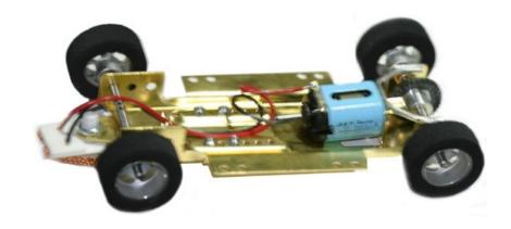
H&R Racing Products Adjustable Wheelbase 1/24 RTR assembled Rolling Chassis - Wheelbase adjustable from 3 5/8" to 4 7/8" (92mm to 123mm) - Includes Hawk 18,000RPM Motor, narrow Foam Rubber 27x12mm tires all around on setscrew aluminum hubs, Oilite bushings, body mounting kit - Comes with inline motor mount & 48 Pitch Cox axle gearing.
