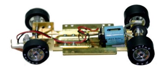
H&R Racing Products Adjustable Wheelbase 1/24 RTR assembled Rolling Chassis - Wheelbase adjustable from 3 5/8" to 4 7/8" (92mm to 123mm) - Includes 18,000 RPM small can Hawk motor, 27x18mm rear Silicone Rubber Rear Tires with 6 Spoke Silver Wheels on setscrew aluminum hubs and rubber tire 6 spoke silver Wheel fronts, Oilite bushings, body mounting kit - Comes with inline motor mount & 48 pitch Cox axle gearing .
